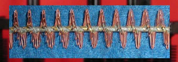
In this type of a turbulator, Wire fins are soldered to a solid center rod. The turbulator is then soldered to the inner surface of the tubes. These "Turbulated Tubes" then can be finned on the outside using any desired type of fins like Wire Wound, Crimped, L, LL, KL etc. Needless to say the soldering of the turbulator and the tubes provides a superior bond giving in turn a larger tube side heat transfer area in addition to turbulation.
