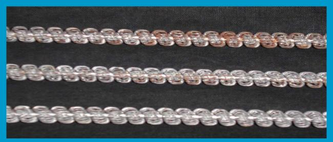
In these turbulators, fins are soldered to a rigid central rod. These turbulators can be then inserted / soldered inside the tubes. These tubes then can be finned (If required) on the outside using any appropriate type of fin. If the turbulator is soldered inside the tubes, the bonding provides superior heat transfer to the tubes.
